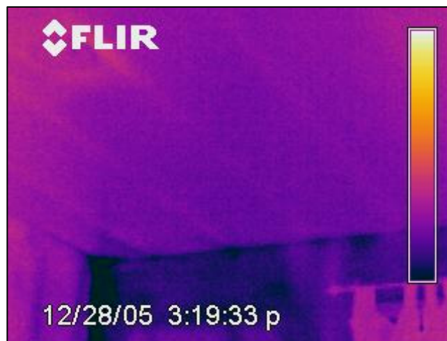
Figure 2.6.2 - Cold air thermal bypass at a porch roof
